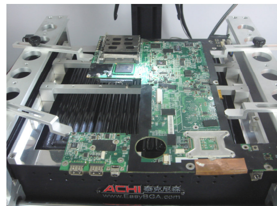
Fixed pole for Shaped Board
